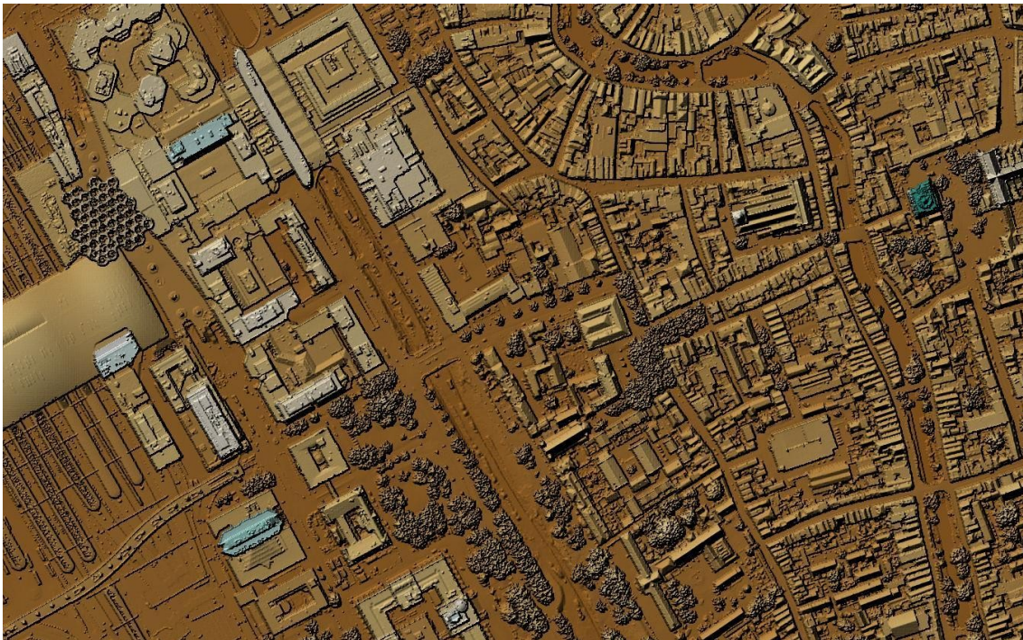
Figure 4: Digital Surface Model (DSM) op basis van AHN4
